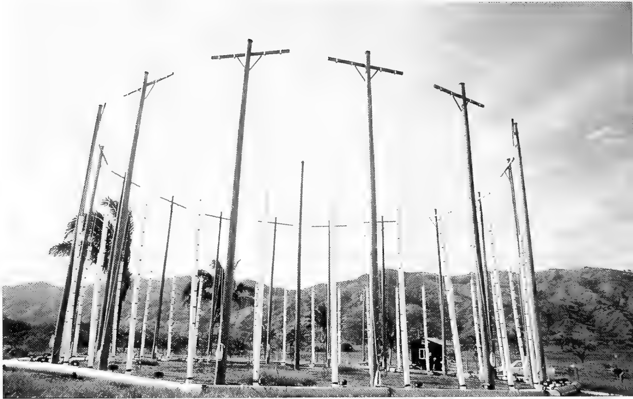
A successful test run of the Free Air Carbon Dioxide Enrichment Ring Project was conducted in Sardinilla in central Panama to study the effects of increased atmospheric carbon dioxide on forest regeneration. The project is a collaborative effort of the Smithsonian Tropical Research Institute, McGill University, Brookhaven National Laboratories of the Department of Energy, the University of Panama, and the Universidad Santa Maria La Antigua. (Photograph by Marcos Guerra)
